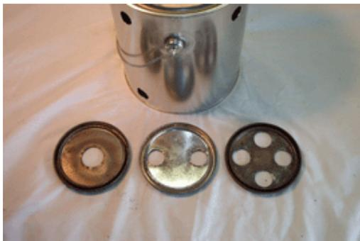
**STEP 8. Extinguish the stove.** Remove the cooking pot from the stove. Using a pair of long nose pliers remove a few support grills. Using the pliers again grab the lip of the quart can lid and carefully place it over the burner, smothering the flame. Wait a while allowing the stove to cool down before touching the stove.
