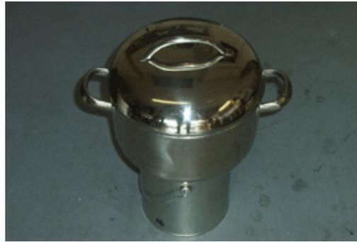
**STEP 7. Adjust the flame.** You can control the flame by placing the lid for the quart paint can (before igniting) half way over the opening. Using a long stick or screw driver slide the lid back and forth over the burner opening to adjust the flame.
