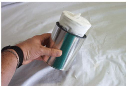
**STEP 5. Add Fuel.** Slowly pour denatured alcohol into the quart paint can. Note: the toilet paper acts as a giant wick and will slow the burning of the alcohol, conserving your fuel. Let the fuel soak into the toilet paper. Continue filling until a small puddle remains just above the top of the toilet paper. Once filled this stove will give you hours of cooking before you need to refill.
