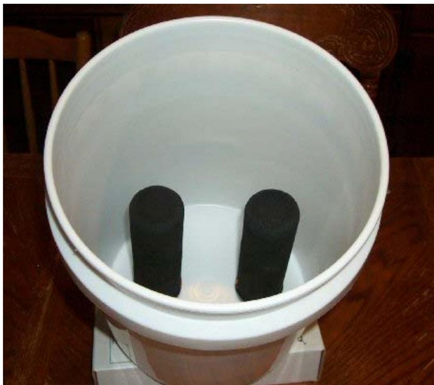
Assemble the filter by placing the upper bucket on the lower. Be sure to line up the holes so the tubes extend through the lid of the lower bucket. Place the remaining lid on top.
