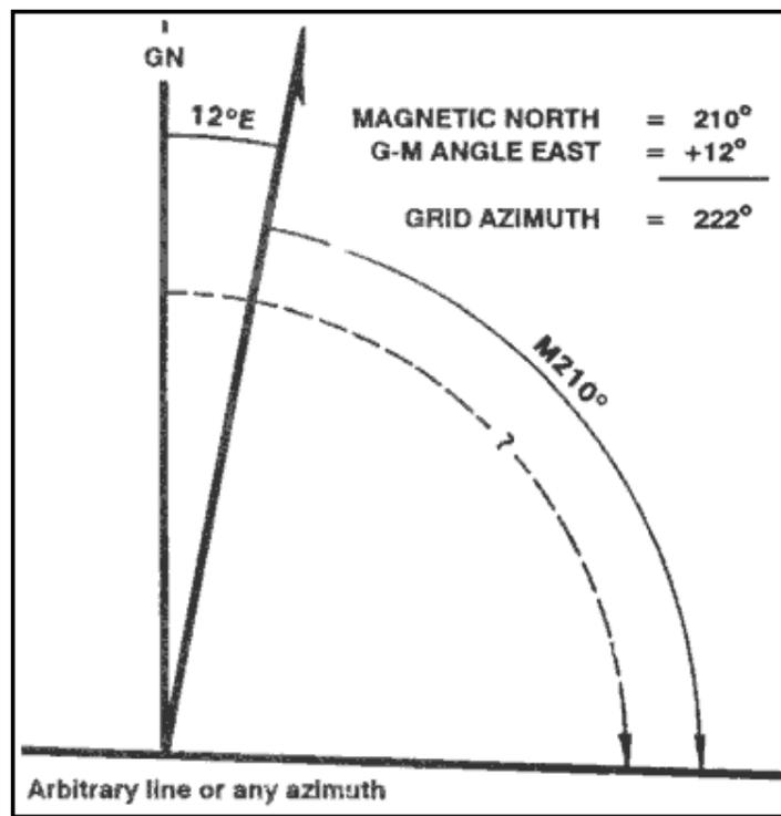
**Figure 6-10. Converting to grid azimuth.**
