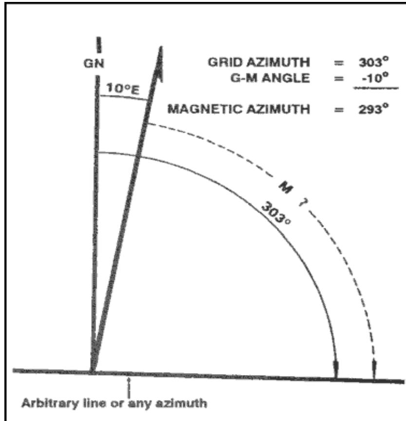
**Figure 6-11. Converting to magnetic azimuth.**
